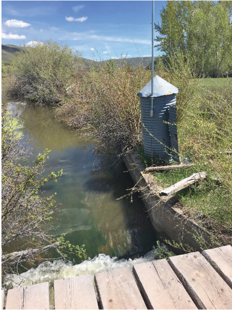
Site 1, 10' steel corrugated stilling well
