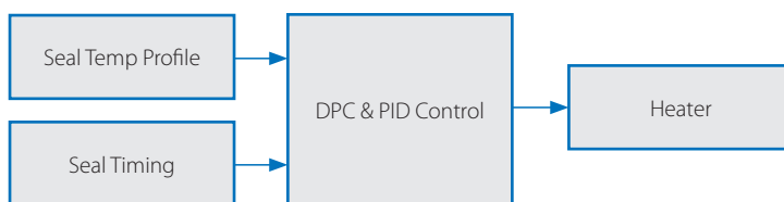
Figure 4. Functional diagram of DPC interaction with PID
